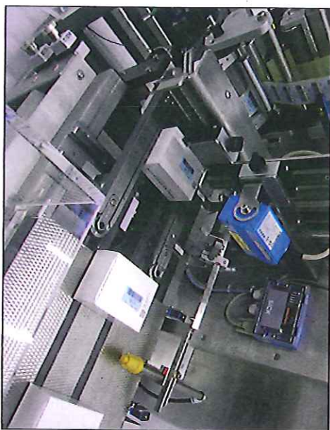
Bosch's CPS 1900 with Labeler is able to print and verify up to 350 cartons per minute and has an integrated labeler.
